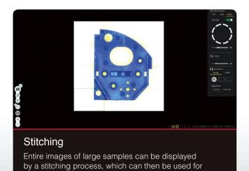
measurement. (\*stitching: bonding of multiple images)
